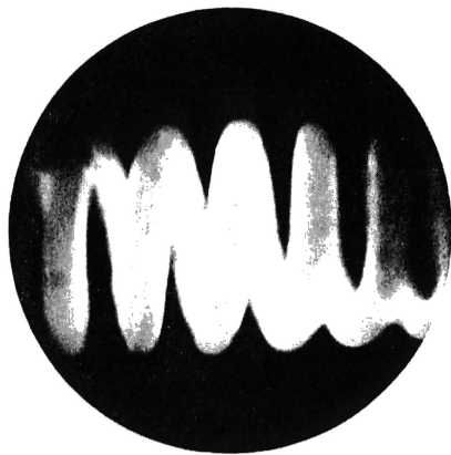
Figure 25: Lamp filament in the lamp-centering device
